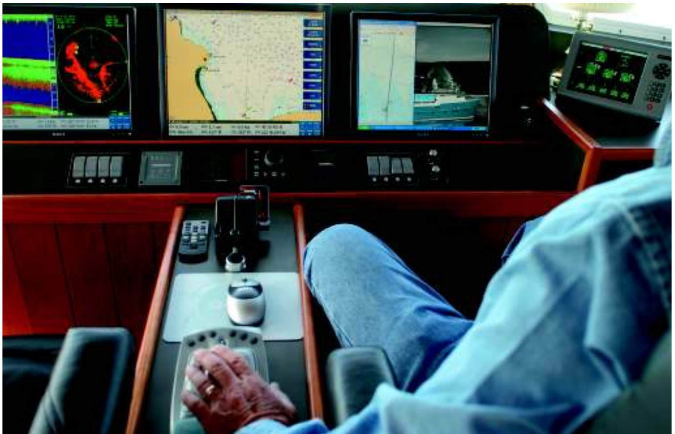
Top: A big mouse, joystick, and engine controller fit neatly on Sonata's console. She doesn't have, or need, a steering wheel. Middle: A Krill Systems, Inc., display offers information on almost every system on board. This screen reports on the status of Sonata's electrical system. Above: The console between helm seats gives left-handed Lee easy use of engine controls and computers. The seats were purchased from a supplier of truck accessories.
